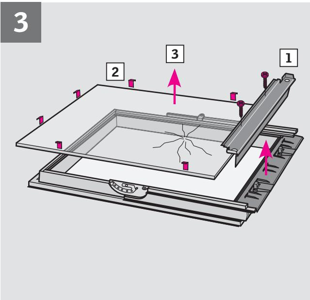
**ENGLISH:** Remove bottom sash cover [1] and distance blocks if fitted [2], then lift out insulating glass unit [3].
