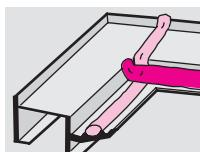
**ENGLISH:** Clean sash profile with methylated spirit. Place thick adhesive sealant strip as shown and press lightly to make it adhere **[1], [2]**. Do not touch adhesive side of strip. Remove cover tape.
