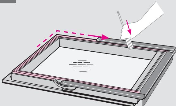
**ENGLISH:** Press sash profile onto insulating glass unit, eg with the handle of a screwdriver.
