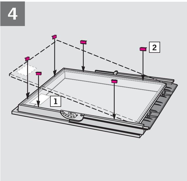
**ENGLISH:** Place insulating glass unit in sash as stated on label **1**. Refit distance blocks if removed earlier **2**. Clean a 50 mm wide area along edge of pane with methylated spirit **3**.
