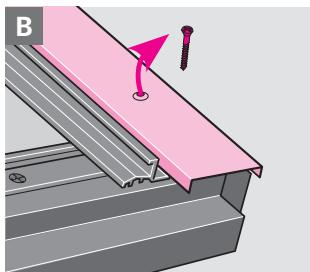
**ENGLISH:** Remove sash covers **1** and sash profile **2** carefully from insulating glass unit. Sash covers may be fixed at the bottom either with brackets **A** or screws **B**.
